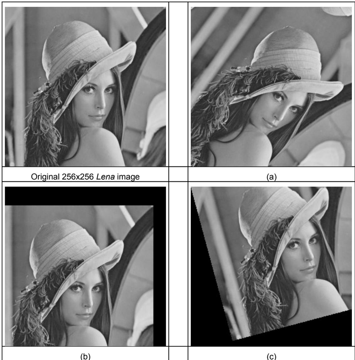
**Figure 6: Some examples illustrating the use of FreeImage\_RotateEx.**
