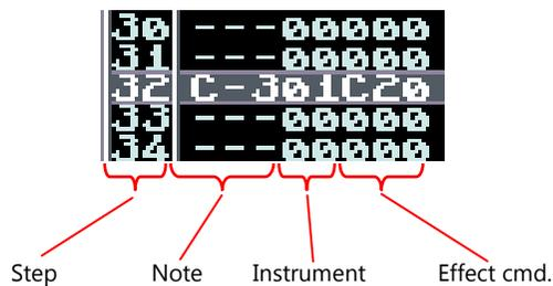
**C-3** is the note being played at track step **32**. **01** is the instrument number, and the last three digits are for the effect command; in this case, **set volume** to **\$20**. **C** is the command, **20** is its value).
